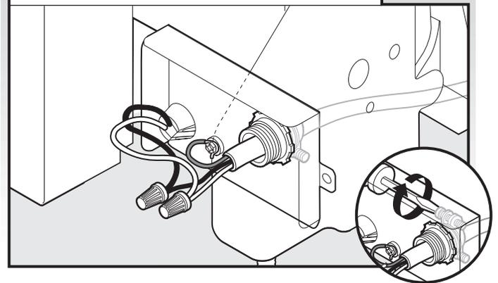
Tighten strain relief screws to secure cable.
